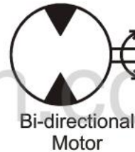
Figure 2-15 A circle with energy triangles symbolize a pump or motor
