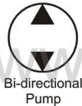
Figure 2-15 A circle with energy triangles symbolize a pump or motor
