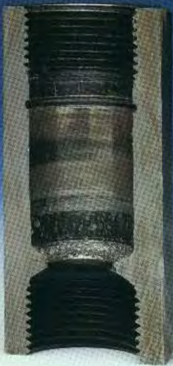
Fig. 240: Seat of a check valve ruined by foreign bodies
