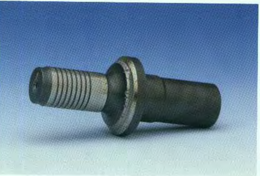
Fig. 239: Erosion of the seat of the pilot cone of a pre-fill valve caused by a very high pressure drop and excessive solids in the fluid
