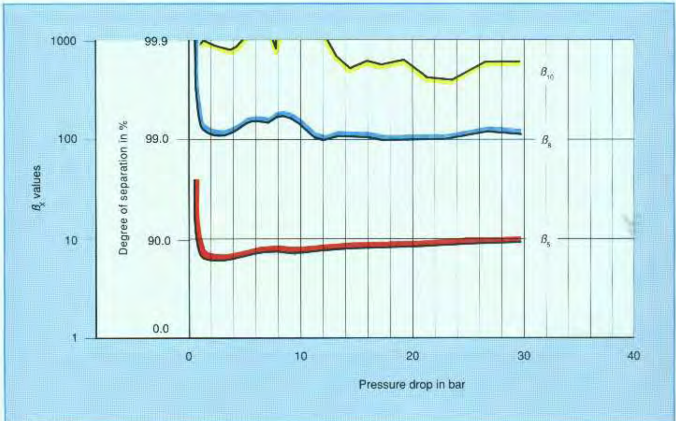
Diagram 38: \beta_x values for different pressure drops across the filter element
