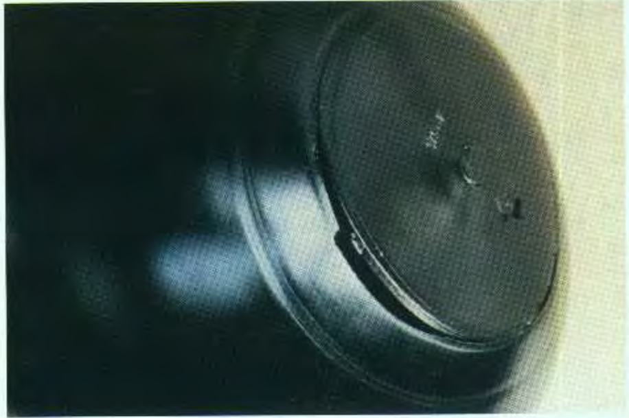
Fig. 246: Torn accumulator bladder. Cause: An excessive fluid flow rate pulled the bladder under the valve plate
