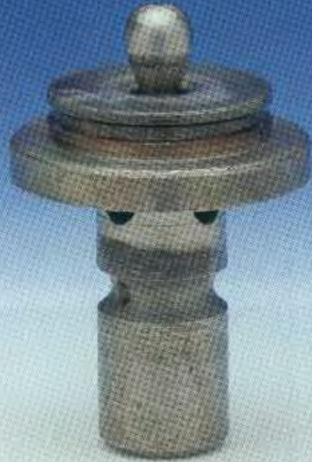
Fig. 241: Normal wear of the cone of a direct-operated pressure relief valve operating very frequently and after a long service life
