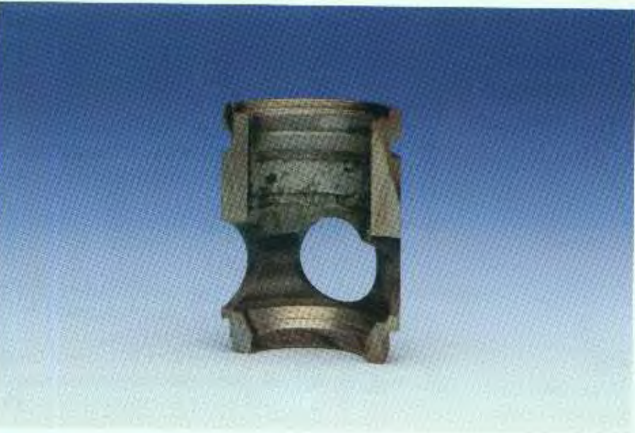
Fig. 238 Traces of seizure between spool and bush of a pilot-operated pressure relief valve. Cause: High-frequency, low-amplitude vibration
