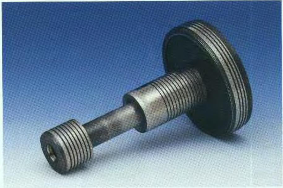
Fig. 247: Worn control land on the piston of a pilot- operated pressure relief valve caused by excessive solids in the fluid
