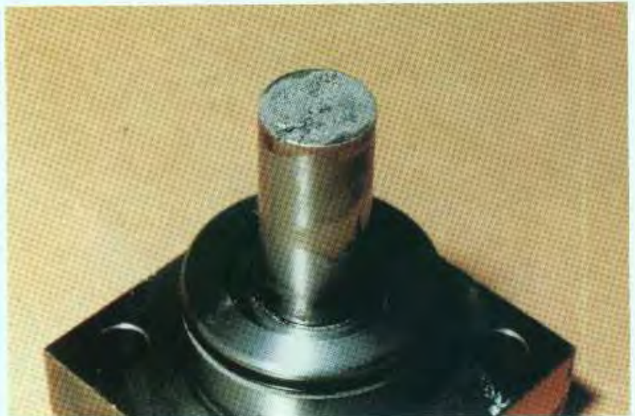
Fig. 242: Cavitation damage to a throttle screw. Remedy: Increased downstream pressure
