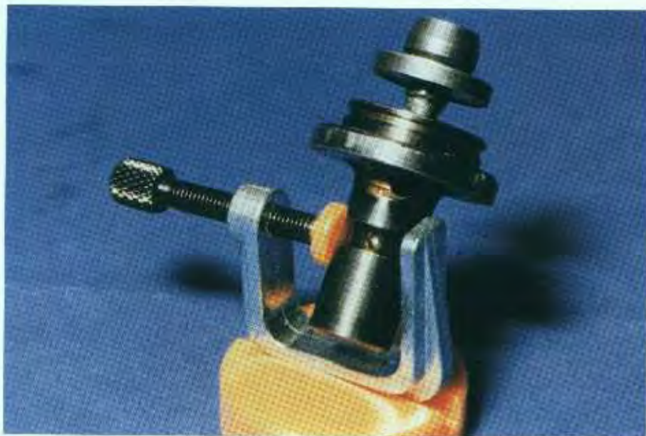
Fig. 243: Erosion of the cone of a direct-operated pressure relief valve. Cause: High pressure drop and high solids content in the fluid combined with frequent operation
