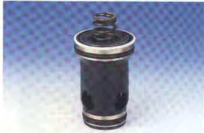
Fig. 1: 2-way cartridge valve (logic element) consisting of a bush, a control poppet and a spring.
