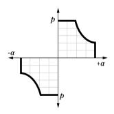
**Basic setting** for design without short circuit valve, de-energized proportional valve and connected control pressure:  $V_{\rm g\ max}$  (see table).
