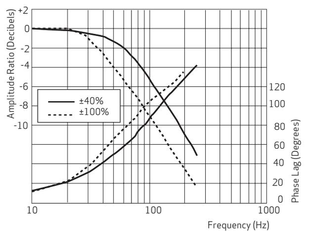
Measured with system pressure  $p_p$  of 210 bar (3,000 psi), oil viscosity 32 mm<sup>2</sup>/s and oil temperature +40 °C (+104 °F)
