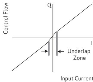
Normally used in hydraulic motor applications
